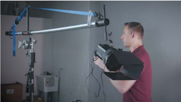
Grip Rigs (19:09) Students learn how to safely build a menace arm and goalpost rig - two common rigs often used on set to place lights in the desired position.
